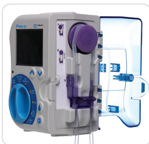
Seat purple cassette into pump. Firmly press the tubing to ensure it is fully seated in slots below the cassette.
